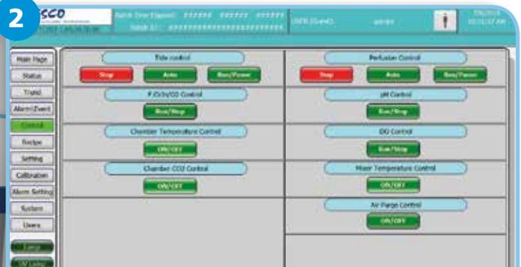
Input the parameters in the TideXcell® system for the inoculation phase and run the program.
