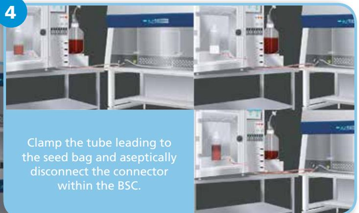
Clamp the tube leading to the seed bag and aseptically disconnect the connector within the BSC.
