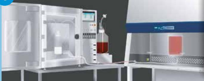
Viral seed or seed cells are prepared in a cGMP Grade B cell/viral processing room with installed CO<sub>2</sub> incubators and Grade A biosafety cabinet (BSC) or a Grade A isolator incubator connected directly to TideXcell® in Grade D background.
