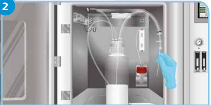
2 Once the sampling tube had reached the end of the tubing, seal the tube with a sealer.
