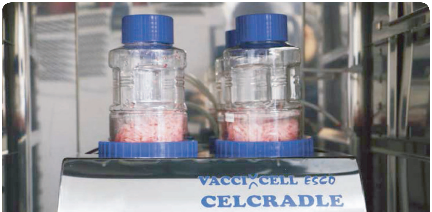
Figure 5: CelCradle-500AP: high cell density was achieved in 3D culturing compared to 2D culturing
