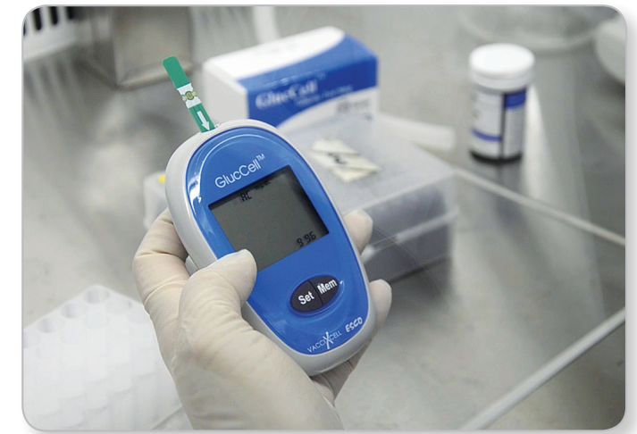
Fig. 2: Portable meter and disposable test strips enable the operation in a biosafety cabinet.
