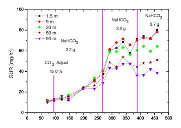
Lower bottom holding time (B\_H) got higher glucose uptake rate. Bottom holding time at below 9 mins did not show any sign of nutrient restriction. B\_H at 30 mins shows nutrient restriction when GUR reach 60 mg/hr; B\_H at 60 and 90 mins show nutrient restriction when GUR reaches around 30 mg/hr.
