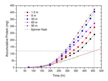
Total harvest IgG in CelCradle-500 in the highest one is 3.3 folds increased compared with a 500 ml spinner flask within 15 days culture period; 3.5 folds increase within 20 days culture and forecast to 4.5 folds increase within a month. With the same working volume, production in spinner flask with 500 ml working volume will require at least 48 days to approach the same IgG production as that in CelCradle in 20 days.
