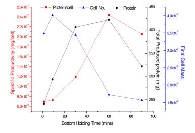
The figure shows that cell growth is reverse proportional to specific productivity. Higher growth rate results lower productivity. The best bottom holding time setting for the best outcome of IgG production will then locate between 30 mins to 60 mins.
